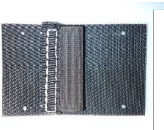
2.5 Stitch Elastic Keeper onto TYPE 12 Webbing as shown. Use Nylon E Thread
