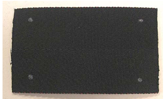
Type XII 75 mm worked with template #1B without drilling the webbing
