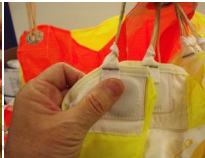
Fig. 10. Check the knot orientation line to fix the knot.
