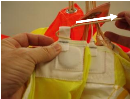
Fig. 9. Apply tension on the C1 line to fix the knot.
