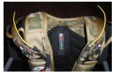
2. Ensure that the release handle is installed; Velcro mated and is all the way up to the top of the inside of the pocket.
