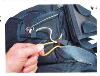
STEP 2. Slide the reserve riser to the outboard side then completely remove the RSL lanyard from its channel beneath the reserve risers. (Fig. 2)
