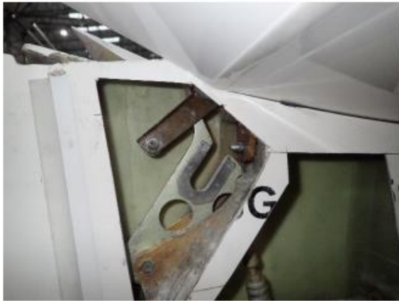
Disconnected elevator control
