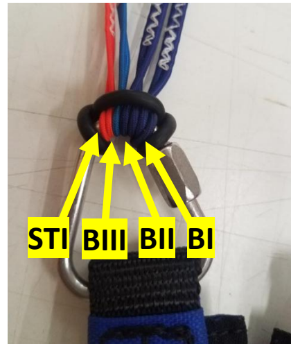
After: BI and BII have 1 trim loops BIII has 0 trim loops, STI has 1 trim loop
